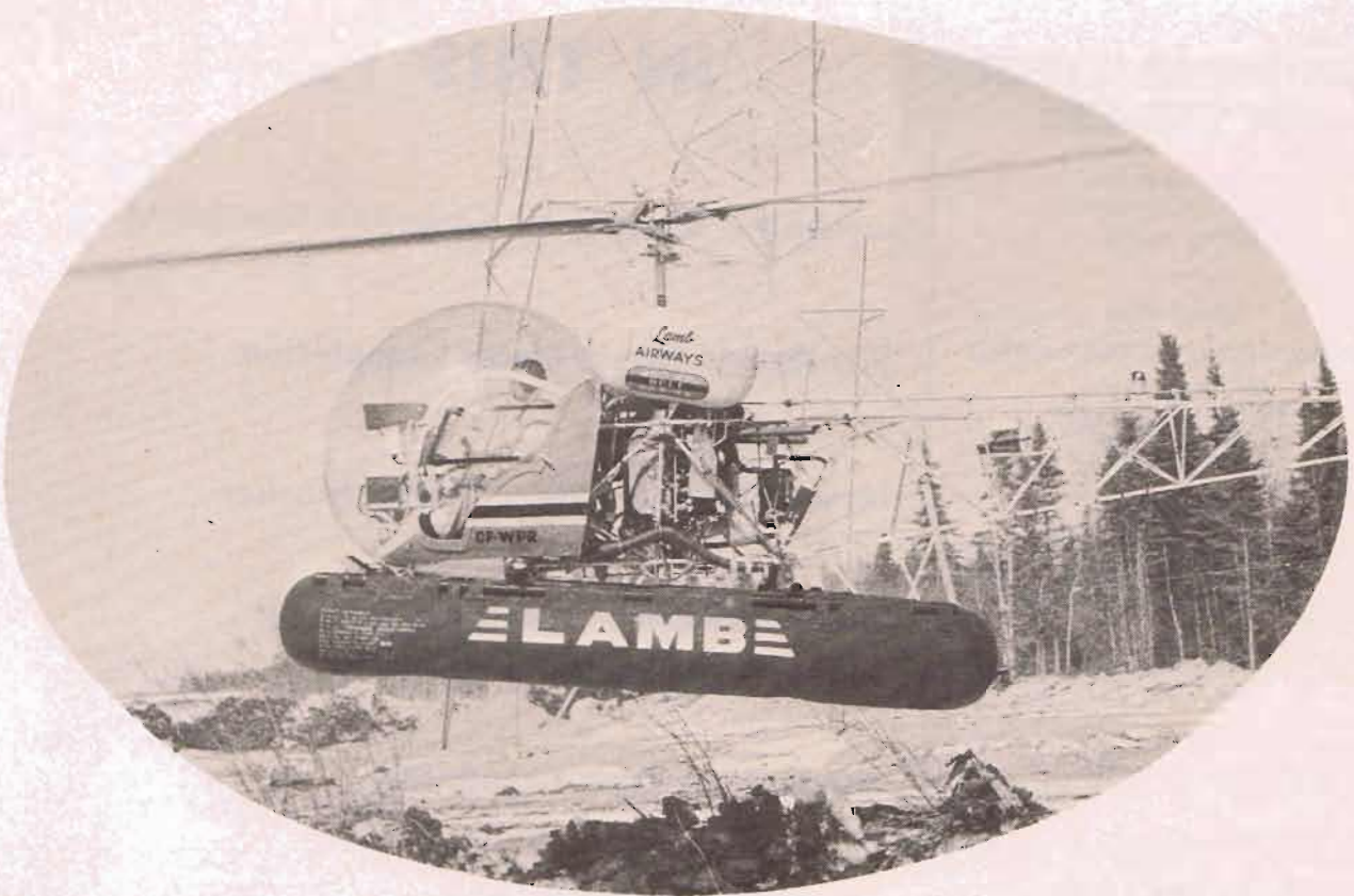
A Bell 47G4A, one of three owned by Lambair. Used mainly on hydro and highway surveys, the aircraft will carry two passengers or 700 pounds payload.
