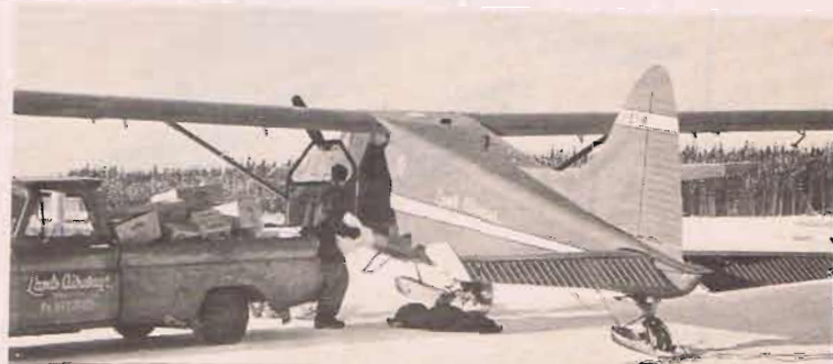
This Beaver aircraft, with a 450 h.p. Pratt Whitney engine, will carry a payload of 1,600 pounds.
