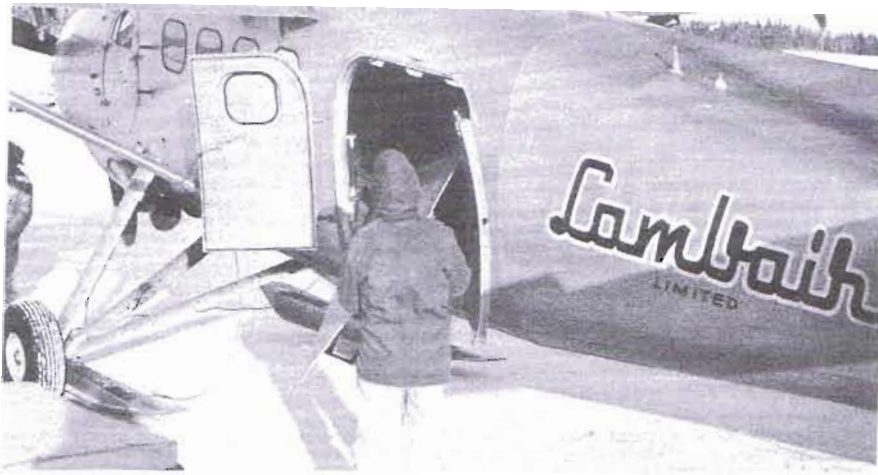
This Otter, with a 600 h.p. Pratt Whitney engine, will carry a payload of one ton.
